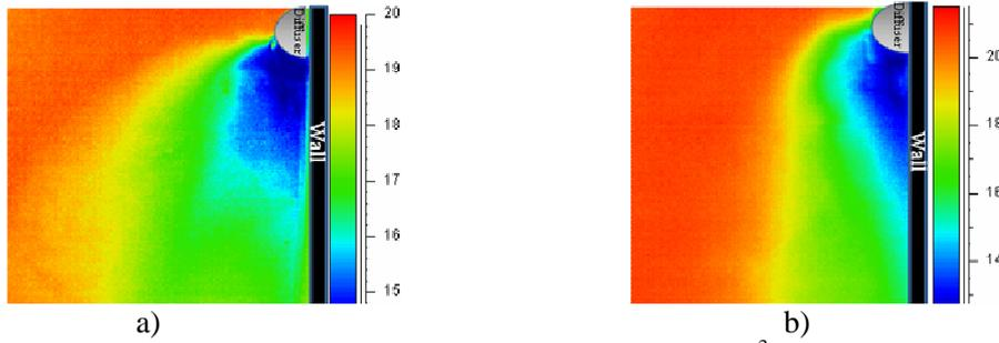
Figure 2. Infrared camera images (a) Airflow rate  $0.040 \text{ m}^3/\text{s}$ ,  $T_{\text{in}} = 15^\circ\text{C}$ , and (b) airflow rate  $0.025 \text{ m}^3/\text{s}$ ,  $T_{\text{in}} = 12.5^\circ\text{C}$ .
