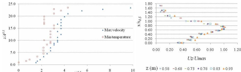
Figure 3. (a) Velocity and temperature trajectory and (b) Non-dimensional mean velocity and temperature profiles in normal direction to the wall at different down-stream locations for Case A.
