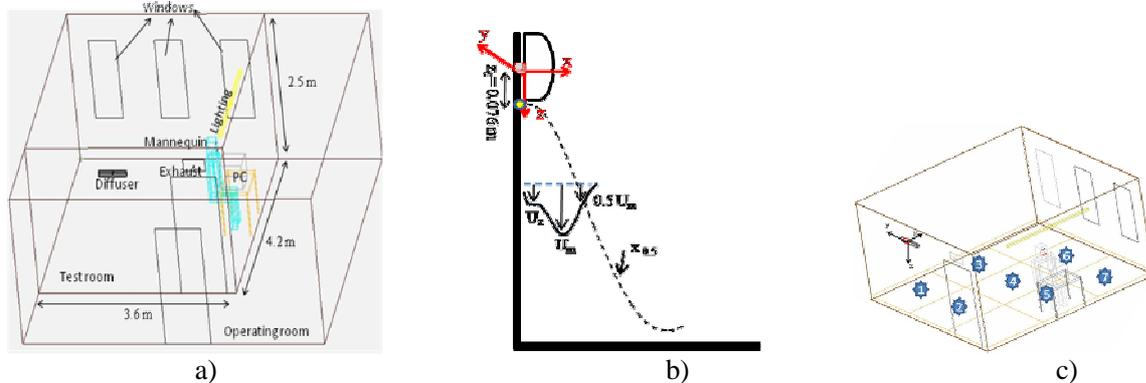
Figure 1. a) Test room layout, b) flow pattern below the diffuser, c) position of the measuring points in the occupied zones.
