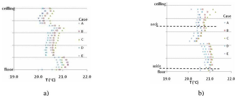
Figure 4. Temperature gradient, a) wall, b) room
