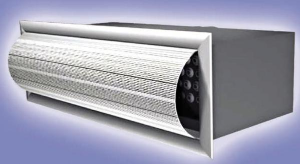
S 55 normally gives double the air exchange efficiency than that from traditional displacement supply air diffusers. Furthermore, the thermal comfort in the room will be significantly improved, as the velocity of the supply air never exceeds 0.2 m/s in the occupied zone.
